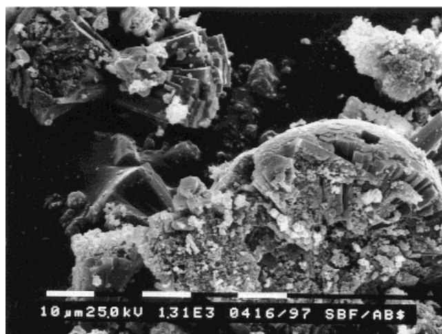
Figure 4. Hydroxyapatite crystallized from simulated body fluid over 26 days (37 °C, unbuffered environment, pH about 7). The polyglycolide matrix was removed by heating to 500 °C; a) interlinked hexagonal prisms that assume terrace-shaped morphology (magnification: \times 5200 ); b) spherical aggregates that have grown out of elongated hexagonal prisms (right); a younger aggregate is visible in the upper left part (magnification: \times 1310 ).
